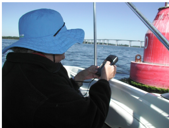
Squadron Member Taking a GPS Fix of a Navigation Buoy for Cooperative Charting
