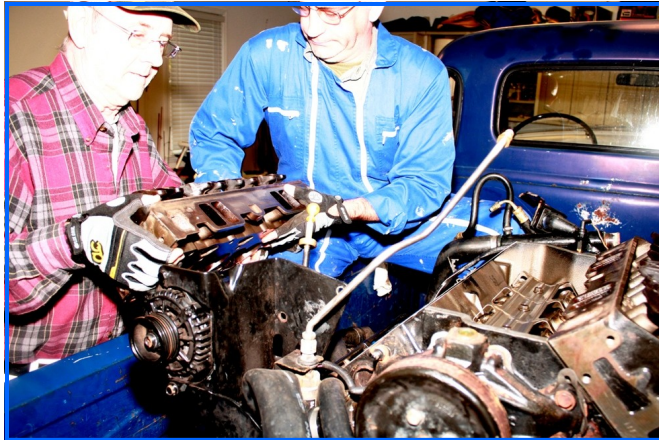
Ted and Scott Erskine Remove the Engine Head
