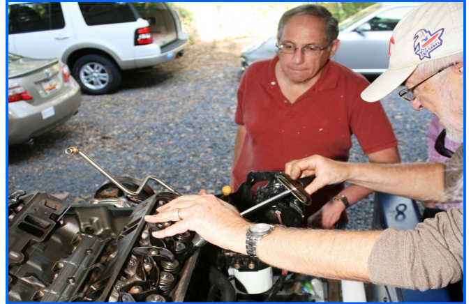
Joel Green Watches Joe Rubin Use Torque Wrench to Tighten Head Bolts
